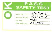
If a brand-new appliance is put into service, it will not be PAT tested initially, instead it will be labelled as in the example below identifying the year in which it can be used before a PAT test is required.
