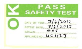
The fields are straightforward, the "DATE OF TEST" is the date of the electrical test, the "RETEST DATE" is set as thirteen months later. This is the crucial date. If this date has passed the appliance must be set aside until it can be retested.
